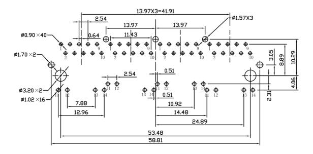
$\label{eq:Suggested} Suggested\ PCB\ Layout\ (Top\ View)$  Dimensions are in millimeters with the following tolerances: X.XX =  $\pm 0.10$
