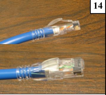
Inspect the terminated plug. Test the completed cable assembly to assure electrical performance meets your requirements.
