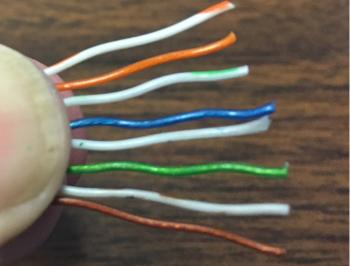
Straighten the wires and arrange them in the proper order.
