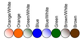
Align wires to standard T568B as shown above.
