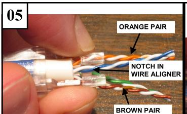
Keep the boot anti-snag toward the rear. Orient the **Orange** pair up and the **Brown** pair down.
