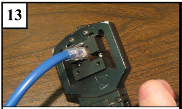
Insert the plug assembly into the crimp tool until it latches. Fully depress the handles to seat the contacts and set the strain relief latch. Crimp tool will open when the termination is complete and pressure is released.
