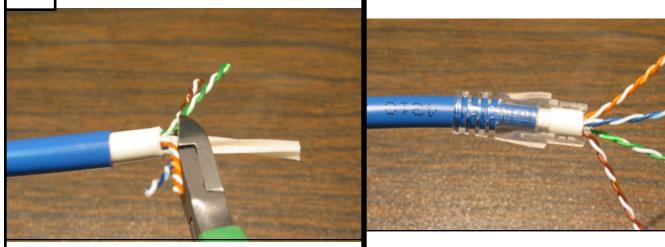
Carefully cut away any spline or any filler strips from the end of the cable. Cut as close as you can to the edge of the jacket without nicking the wire insulation.
