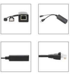
Active PoE splitter separates 5V 1A power to a USB Micro-B plug and 10/100/1000 Mbps Gigabit Ethernet data to an RJ45 plug.
