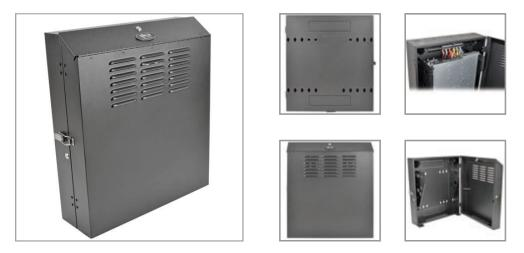
Wall-mount cabinet secures and organizes 4U of 19-inch rack equipment in network wiring closets and other locations with limited floor space. Houses equipment up to 20 inches deep, but extends just 8 inches from wall.
