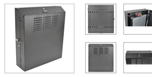
Wall-mount cabinet secures and organizes 6U of 19-inch rack equipment in network wiring closets and other locations with limited floor space. Houses equipment up to 20 inches deep, but extends less than 12 inches from wall.
