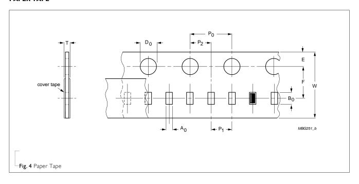
Table 4 Dimensions of paper tape for relevant chip resistors size
