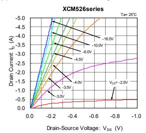
(2) Drain Current vs. Drain Source Voltage
