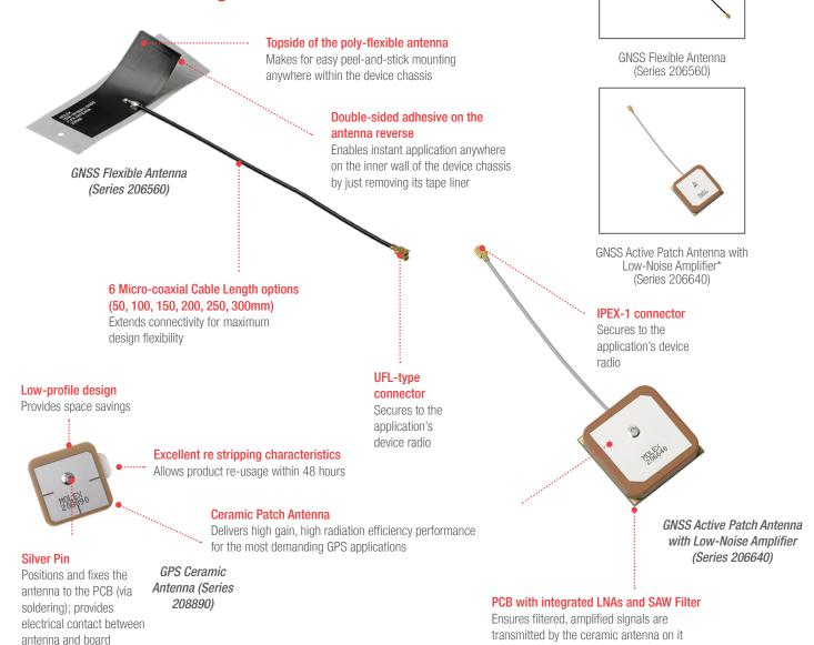
\*The series 206640 antenna is an active patch antenna with ceramic patch, ground plane (PCB), 2-stage LNA and SAW (Surface Acoustic Wave) filter - all integrated within a compact 25 by 25 by 6.5mm module complete with a 60mm cabled (IPEX-1 connector) extension.
