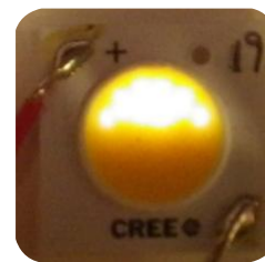
Figure 4: Partially illuminated CX family LED due to damaged bond wires
