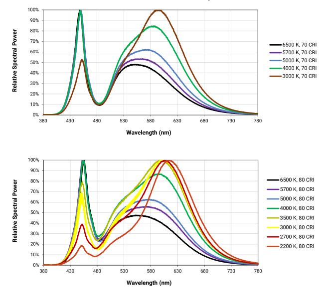
The following graphs are the result of a series of pulsed measurements at 1620 mA and T<sub>1</sub> = 85 °C.
