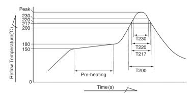
T200 : Duration for over +200  $\!\!\!\!^{\circ}_{\circ}$  at capacitor surface.
