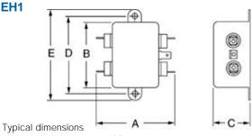
Terminals:  $\frac{.250}{6.35}$ (5) Holes:  $\frac{.0.7}{1.8}$  Dia.(4) Slot:  $\frac{.07 \times .16}{1.8 \times 4.1}$
