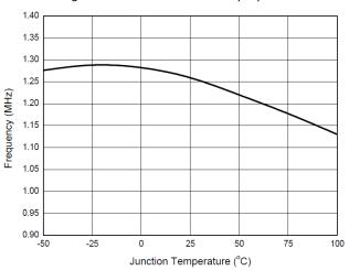
Fig. 12: Switching Frequency vs Junction Temperature
