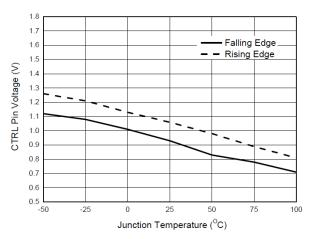
Fig. 16: CTRL Pin Voltage vs. Junction Temperature
