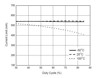
Fig. 10: Current Limit vs. Duty Cycle
