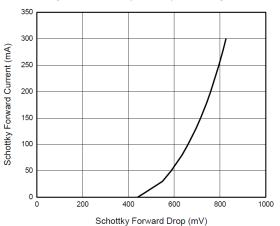
Fig. 7: Schottky Forward Current vs Schottky Forward Drop
