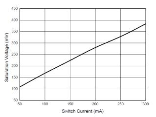
Fig. 17: Switch Saturation Current vs Switch Current
