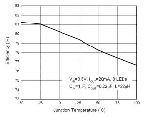
Fig. 4: Efficiency vs. Junction Temperature
