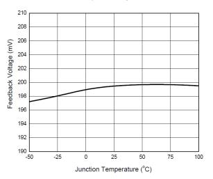
Fig. 13: Feedback Voltage vs Junction Temperature
