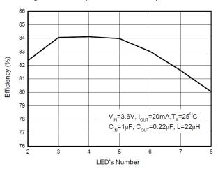
Fig. 6: Efficiency vs. Number of LEDs
