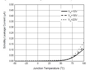
Fig. 15: Schottky Leakage Current vs Junction Temperature
