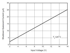
Fig. 8: Shutdown Quiescent Current vs Input Voltage
