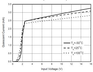
Fig. 9: Supply Current vs Input Voltage
