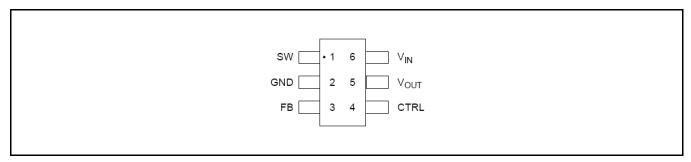
Fig. 3: SP6699 Pin Assignment
