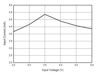
Fig. 11: Input Current in Output Open Circuit vs Input Voltage
