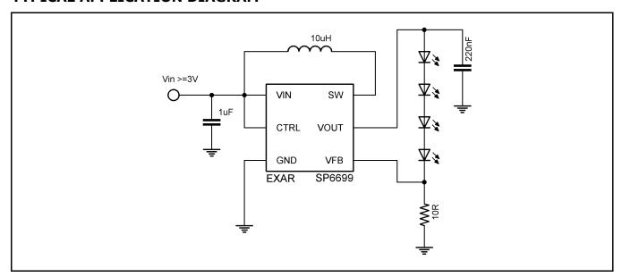
Fig. 1: SP6699 Application Diagram
