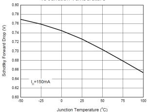
Fig. 14: Schottky Forward Drop vs Junction Temperature
