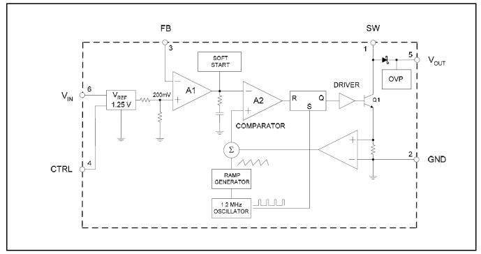
Fig. 2: SP6699 Block Diagram
