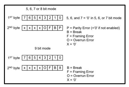
Figure 5: Wide Mode Receive Data Format
