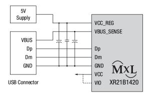
Figure 2: Self-Powered 5V Mode
