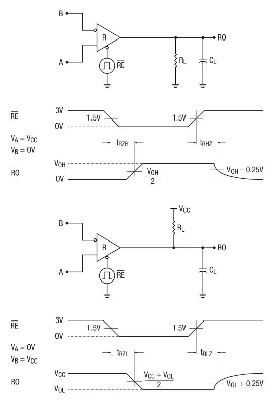
Figure 5. Receiver Enable and Disable Test Circuits and Timing Diagrams
