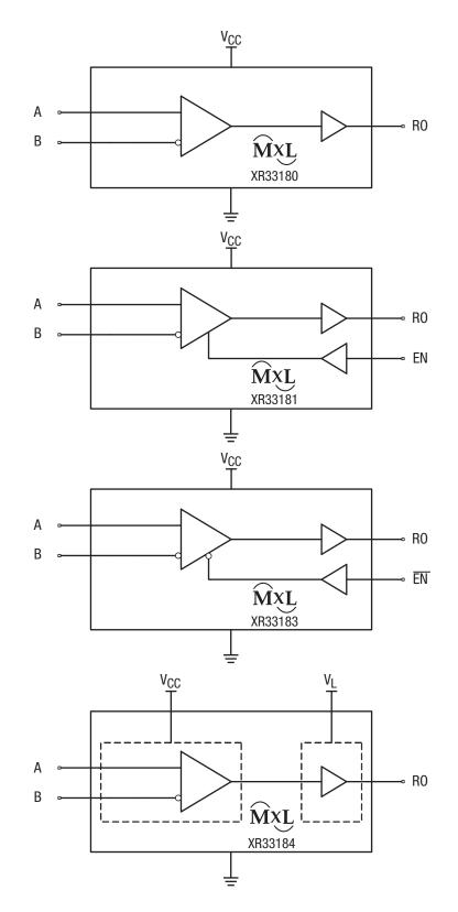
Figure 2. Functional Block Diagrams
