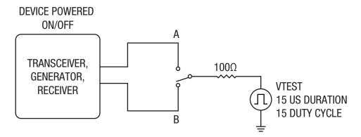
Figure 3. Transient Overvoltage Test Circuit
