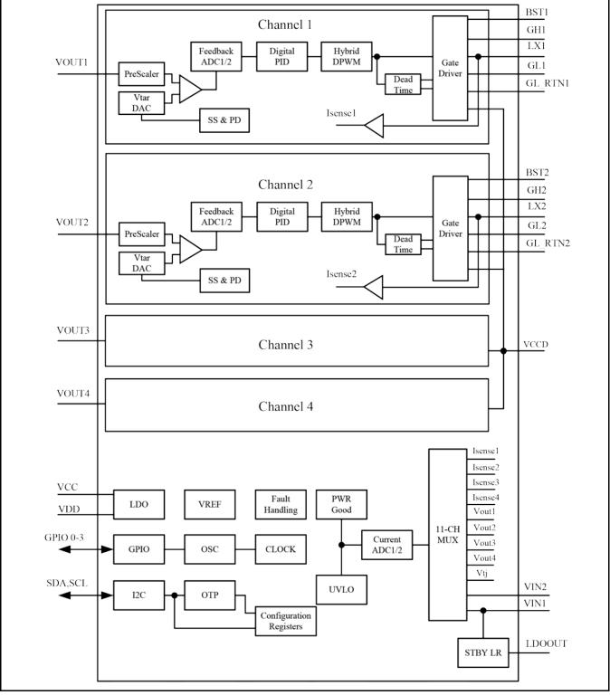
Fig. 2: XRP7714 Block Diagram
