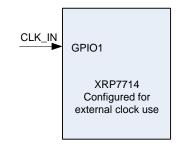
Fig. 27: XRP7714 Configured For External Clock Use
