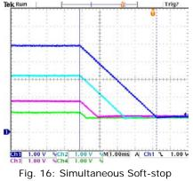
V<sub>OUT</sub> Shutdown=0.8V, 3A load CH1:3.3V, CH2:5V, CH3:1V, CH4:1.8V
