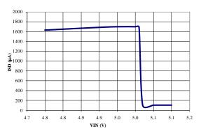
Fig. 11: Shutdown Current 4.8V to 5.1V
