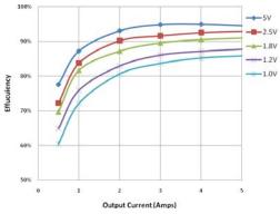
Fig. 4: 12Vin Efficiency: Single Channel 300kHz - Channels not in use are disabled FET: Si4944; Inductor: 744314xxx 7x7x5mm
