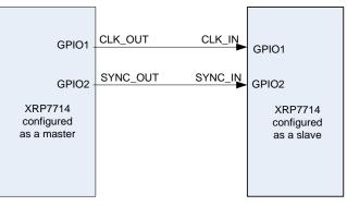
Fig. 28: Master/Slave Configuration of the XRP7714
