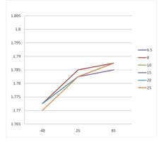
Fig. 20: Temperature and Voltage Regulation 1.8V out (±1% Vout window)
