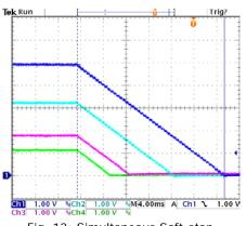
Fig. 13: Simultaneous Soft-stop CH1:3.3V, CH2:5V, CH3:1V, CH4:1.8V
