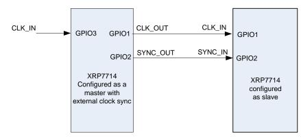
Fig. 30: Alternative External clock synchronization Master Slave combination
