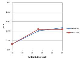
Fig. 19: Temperature Regulation 1.0V out (±1% Vo window)
