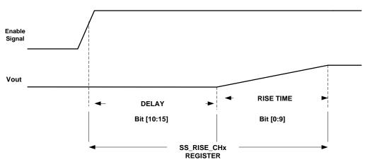
Fig. 24: Channel Power Up Sequence
