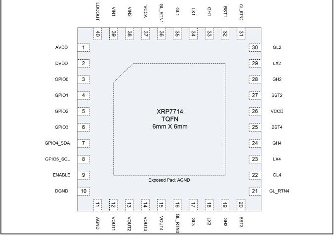
Fig. 3: XRP7714 Pin Assignment
