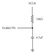
Fig. 21: RC Delay for Enable taken from VCCA
