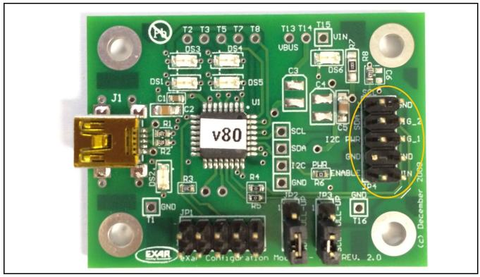
Figure 2: XR77XXEVB-XCM-V80 JP4 Pin Assignment
