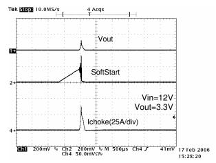
Figure 8. Output Load Short Circuit
