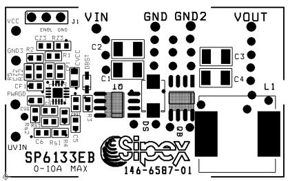
Figure 13. SP6133EB Component Placement
