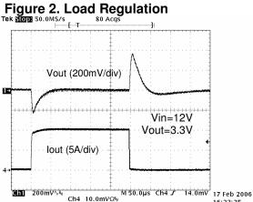
Figure 4. Load Step Response: 0->10A
