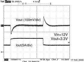
Figure 3. Load Step Response: 5->10A
