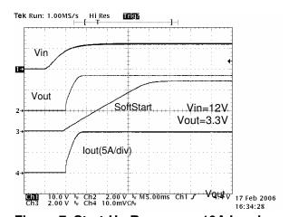
Figure 7. Start-Up Response: 10A Load
