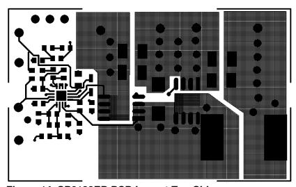
Figure 14. SP6133EB PCB Layout Top Side
