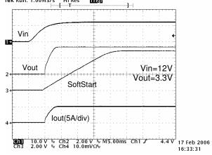
Figure 6. Start-Up Response: 5A Load
