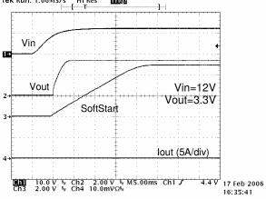
Figure 5. Start-Up Response: No Load
