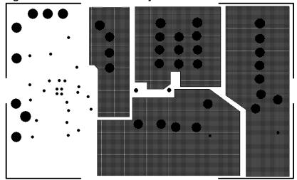
Figure 16. SP6133EB PCB Layout Inner Layer 1 & Inner Layer 2
