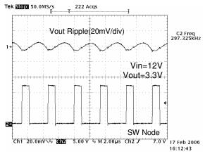
Figure 9. Output Noise at No Load
