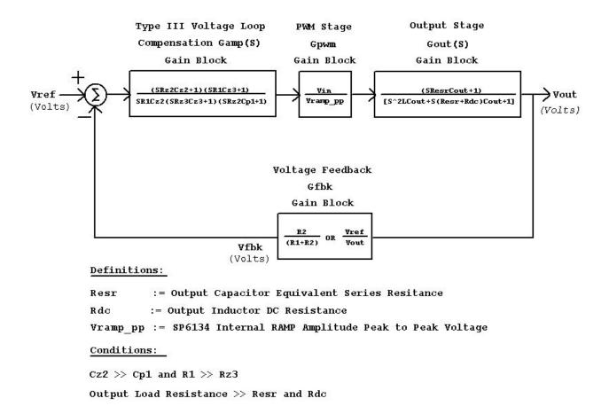
Figure 11. SP6133EB Voltage Mode Control Loop with Loop Dynamic
