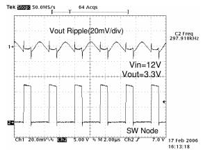
Figure 10. Output Noise at 10A Load
