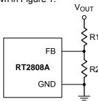
Figure 1. Output Voltage Setting
