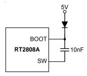
Figure 2. External Bootstrap Diode
