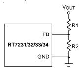
Figure 4. Output Voltage Setting
