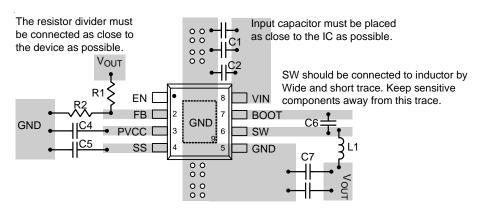
(c). For SOP-8 (Exposed) Package
