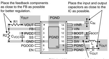
SW should be connected to inductor by Wide and short trace. Keep sensitive components away from this trace.
