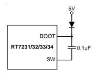
Figure 5. External Bootstrap Diode
