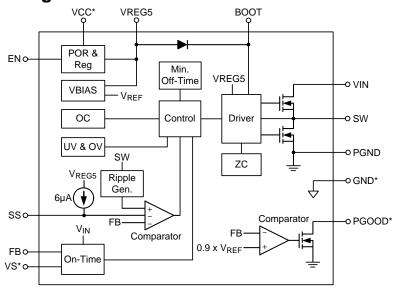
\*: VCC pin for TSSOP-14 (Exposed Pad) only. VS pin for TSSOP-14 (Exposed Pad) only. GND pin for TSSOP-14 (Exposed Pad) only. PGOOD pin for TSSOP-14 (Exposed Pad) and WDFN-10L 3x3 only.
