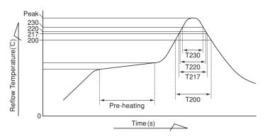
T200: Duration for over +200°C at capacitor surface.
