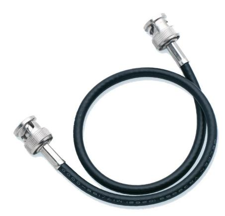
• Mueller's BU-5050-B is a cable assembly with male BNC connectors on each end of an RG-58/U coaxial cable.
