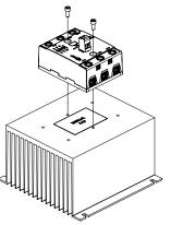
fig.1 SSR mounted on HS053 heat sink
