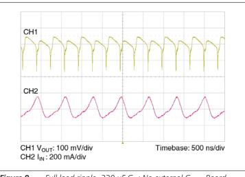
**Figure 9** — Full load ripple, 330 μF C<sub>IN</sub>; No external C<sub>OUT.</sub> Board mounted module, scope setting : 20 MHz analog BW
