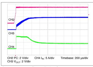
**Figure 10** — Start up from application of PC;  $V_{IN}$  pre-applied  $C_{OUT} = 9100 \ \mu F$
