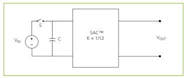
Figure 15 — Sine Amplitude Converter™ with input capacitor
