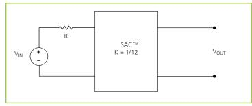
**Figure 14** — K = 1/12 Sine Amplitude Converter™ with series input resistor
