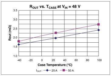
**Figure 7** — R<sub>OUT</sub> vs. temperature
