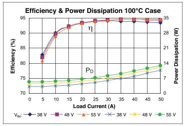
**Figure 6** — Efficiency and power dissipation at  $T_C = 100^{\circ}C$
