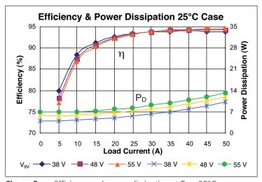
**Figure 5** — Efficiency and power dissipation at  $T_C = 25^{\circ}C$
