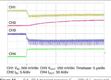
**Figure 11** — 0 A– 50 A transient response:  $C_{IN}$  = 330  $\mu$ F,  $I_{IN}$  measured prior to  $C_{IN}$ , no external  $C_{OUT}$
