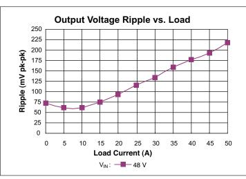
**Figure 8** —  $V_{RIPPLE}$  vs.  $I_{OUT}$ ; No external  $C_{OUT}$ . Board mounted module, scope setting: 20 MHz analog BW
