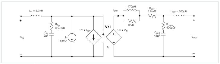
Figure 17 — VI Chip® module AC model
