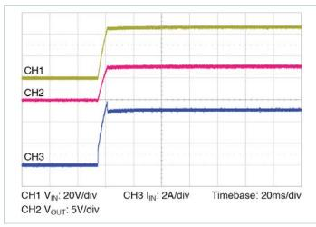
**Figure 13** — Start up from application of  $V_{IN}$ : VC pre-applied  $C_{OUT} = 2300 \mu F$
