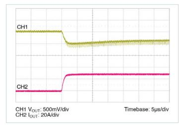
**Figure 15** — OA – Full load transient response:  $C_{IN} = 100 \mu F$ , no external  $C_{OUT}$
