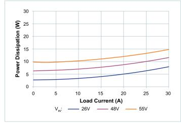
Figure 4 — Power dissipation at -40°C
