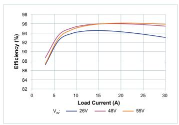
Figure 7 — Efficiency at 100°C
