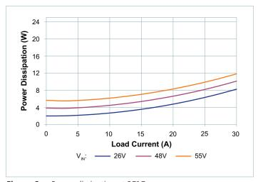
**Figure 6** — Power dissipation at 25°C
