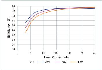
**Figure 3** — Efficiency at −40°C
