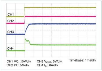
**Figure 14** — Start up from application of VC;  $V_{IN}$  pre-applied  $C_{OUT} = 2300 \mu F$
