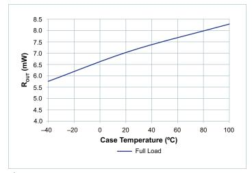
**Figure 9** — R<sub>OUT</sub> vs. temperature
