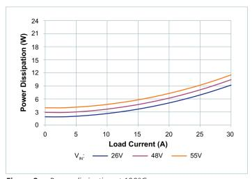
Figure 8 — Power dissipation at 100°C
