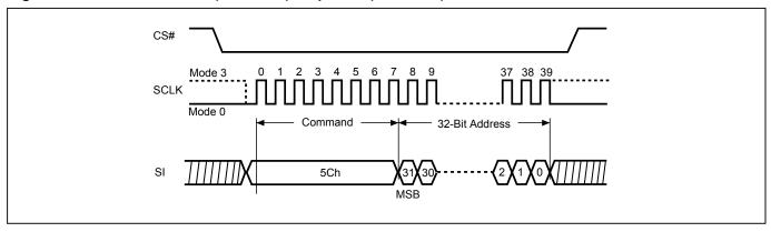
Figure 66. Block Erase (BE4B) Sequence (SPI Mode)
