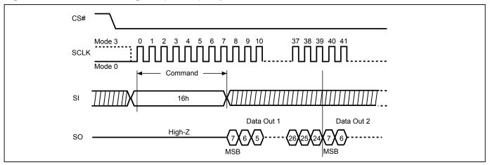
Figure 78. Write Fast Boot Register (WRFBR) Sequence
