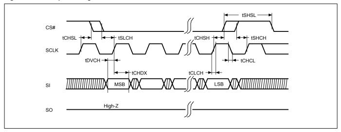
Figure 3. Serial Input Timing (DTR mode)
