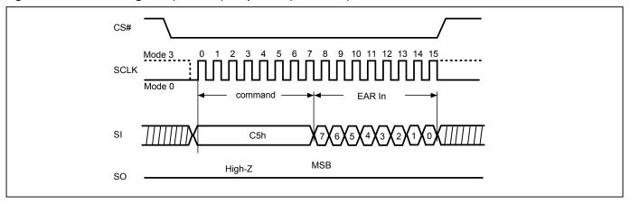
Figure 8. Write EAR Register (WREAR) Sequence (QPI Mode)
