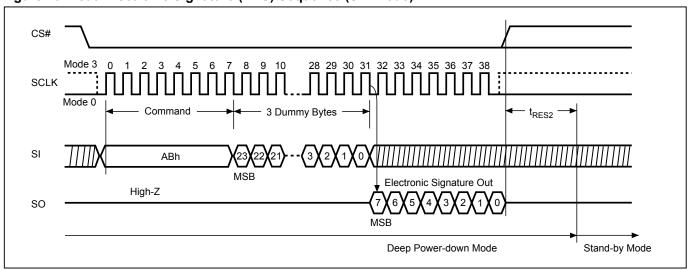
Figure 20. Read Electronic Signature (RES) Sequence (SPI Mode)
