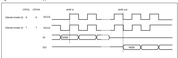
Figure 1. Serial Modes Supported
