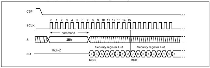
Figure 94. Read Security Register (RDSCUR) Sequence (QPI Mode)
