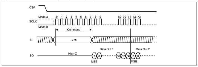
Figure 109. Write Password Register (WRPASS) Sequence
