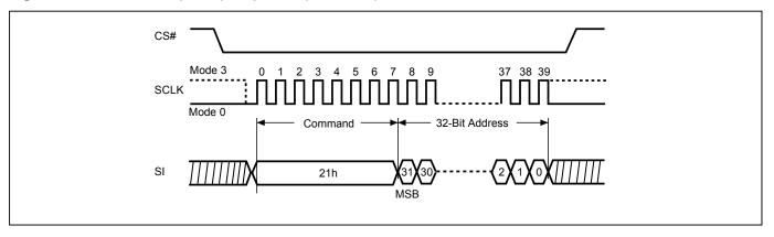
Figure 65. Block Erase 32KB (BE32K4B) Sequence (SPI Mode)
