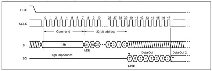
Figure 57. Read Data Bytes at Higher Speed using 4-Byte Address Sequence (FASTREAD4B)
