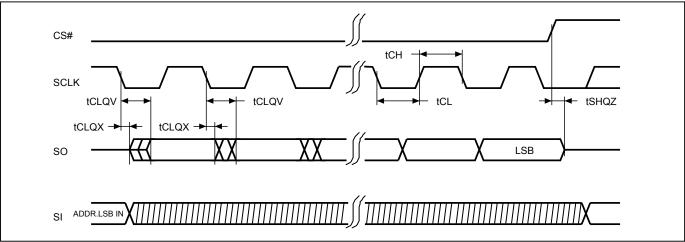
Figure 5. Output Timing (DTR mode)
