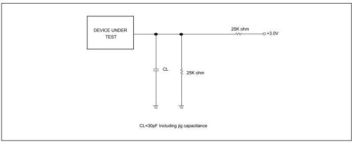
Figure 123. SCLK TIMING DEFINITION
