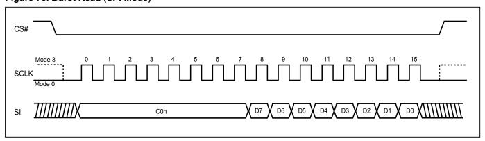
Figure 74. Burst Read (QPI Mode)
