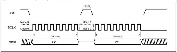
Figure 116. Reset Sequence (QPI mode)
