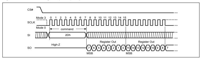
Figure 100. Write Lock Register (WRLR) Sequence (SPI Mode)
