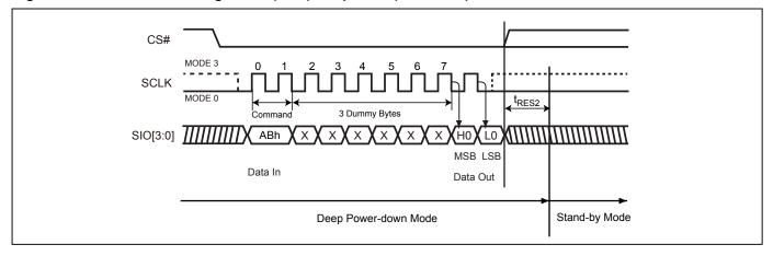
Figure 22. Release from Deep Power-down (RDP) Sequence (SPI Mode)
