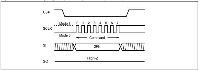
Figure 96. Write Security Register (WRSCUR) Sequence (QPI Mode)
