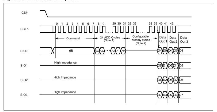
Figure 39. Quad Read Mode Sequence
