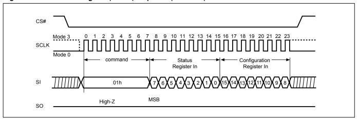
Figure 31. Write Status Register (WRSR) Sequence (SPI Mode)
