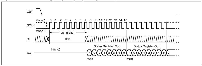
Figure 26. Read Status Register (RDSR) Sequence (QPI Mode)
