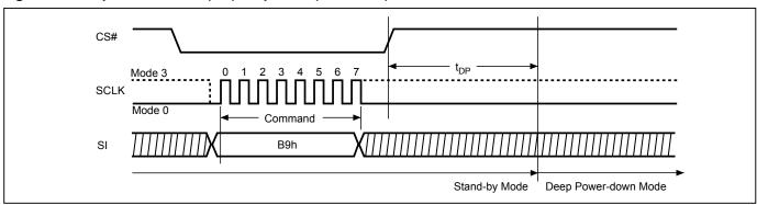
Figure 92. Deep Power-down (DP) Sequence (QPI Mode)
