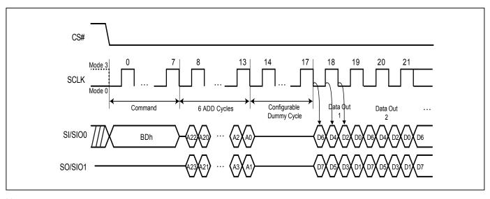
Figure 43. Fast Dual I/O DT Read (2DTRD) Sequence (SPI Only)
