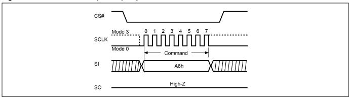
Figure 102. Read SPB Lock Register (RDSPBLK) Sequence
