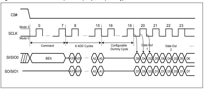
Figure 61. Fast Dual I/O DT Read (2DTRD4B) Sequence (SPI Only)
