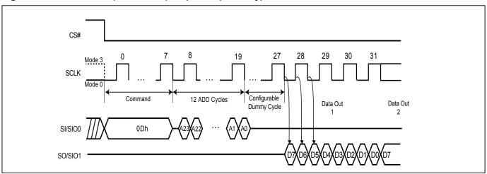
Figure 42. Fast DT Read (FASTDTRD) Sequence (SPI Only)
