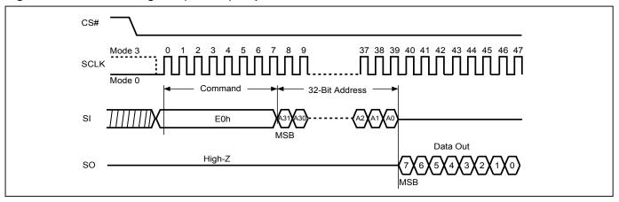
Figure 107. Write DPB Register (WRDPB) Sequence
