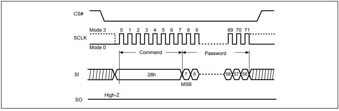
Figure 110. Password Unlock (PASSULK) Sequence
