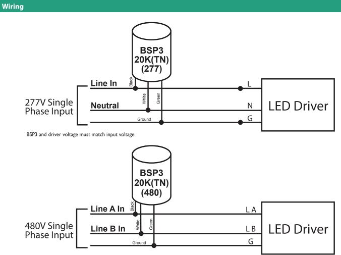
A single phase input from a 3-phase system uses only 2 phase line connections (A-B, B-L or C-A)
