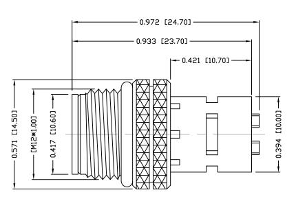
NΠΤF: MATERIAL HOUSING: PBT UL94V-0, BLACK CONTACT: BRASS NUT: BRASS EPDM, BLACK □-RING: SHELL: BRASS FINISH CONTACT: GOLD PLATED □VER 504" NICKEL NUT: NICKEL PLATED SHELL: BRIGHT TIN PLATED **ELECTRICAL** RATED CURRENT: 4A RATED VOLTAGE: 250V INSULATION RESISTANCE: 100 MOhms MIN. CONTACT RESISTANCE: 10 mOhms MAX. IP67 WATER PROOF: **ENVIRONMENT** -40°C TD +85°C **OPERATION TEMPERATURE:** MAX WIRE AWG: 22
