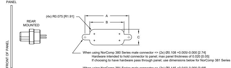
When using NorComp 381 Series male connector => (2x) Ø0.145 +0.010/-0.000 [3.68] Hardware intended to pass through panel
