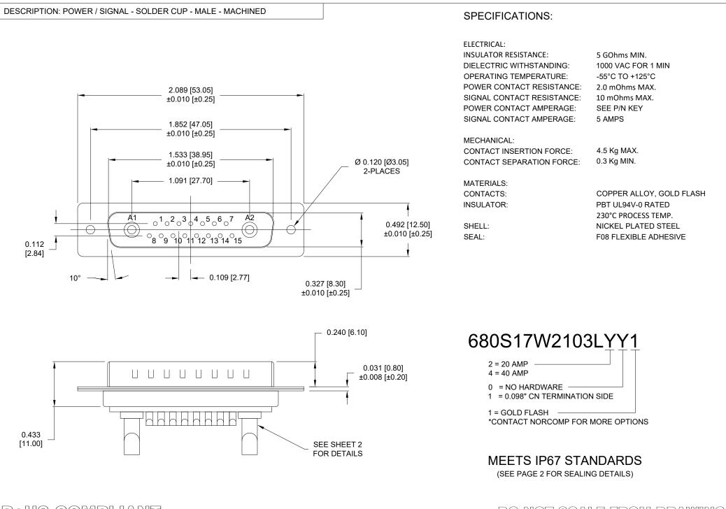
ROHS COMPLIANT DO NOT SCALE FROM DRAWING UNITS = inch [mm] DRAWN: SCALE: SHEET OF M. SIGMON NorComp THE PROPERTY OF NorComp AND SHALL NOT NTS 2 1 DWG NO. DATE: 680S17W2103LYY1 04/03/2012 APPARATUS WITHOUT WRITTEN PERMISSION.
