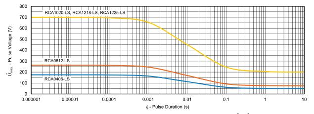
Maximum pulse voltage, single and continuous pulses; applicable if  $\hat{P} \leq \hat{P}_{\text{max.}}$ ; for permissible resistance change equivalent to 8000 h operation
