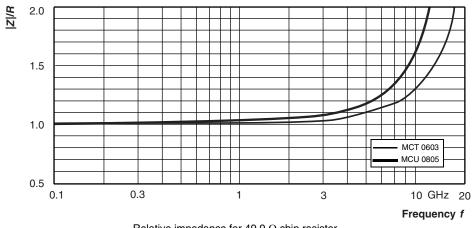
Relative impedance for 49.9  $\Omega$  chip resistor
