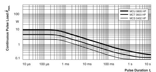
Maximum pulse load, continuous pulses; applicable if  $\overline{P} \leq P$  ( $\vartheta_{amb}$ ) and  $\hat{U} \leq \hat{U}_{max}$ ; for permissible resistance change  $\pm$  (0.5 % R + 0.05  $\Omega$ )
