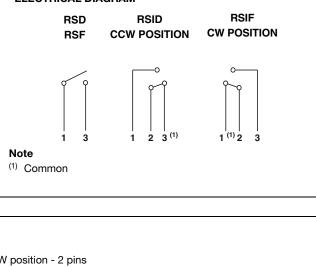
RSDSPST: Single pole, open switch in CCW position - 2 pinsRSFSPST: Single pole, open switch in CW position - 2 pinsRSIDSPDT: Single pole, changeover switch in CCW position - 3 pinsRSIFSPDT: Single pole, changeover switch in CW position - 3 pins
