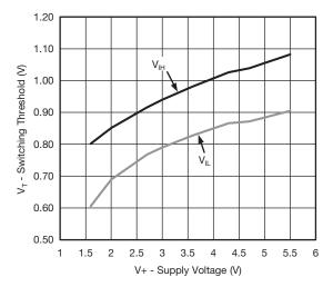
Switching Threshold vs. Supply Voltage
