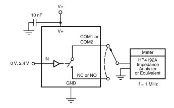
Fig. 5 - Channel Off/On Capacitance
