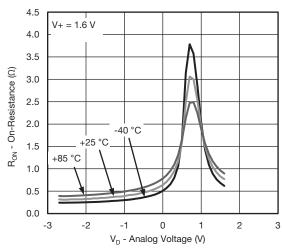
On-Resistance vs. Analog Voltage and Temperature
