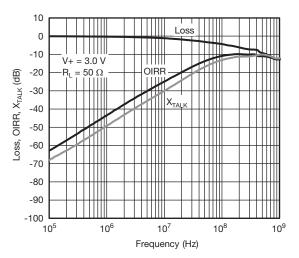
Insertion Loss, Off-Isolation, Crosstalk vs. Frequency
