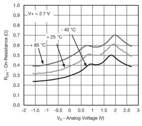
On-Resistance vs. Analog Voltage and Temperature
