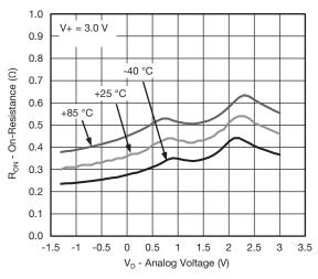
On-Resistance vs. Analog Voltage and Temperature
