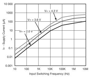
**Supply Current vs. Input Switching Frequency**
