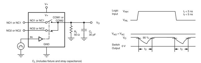
Fig. 2 - Break-Before-Make Interval
