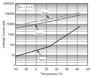
Leakage Current vs. Temperature
