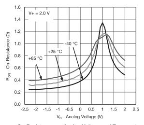
On-Resistance vs. Analog Voltage and Temperature
