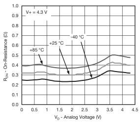
On-Resistance vs. Analog Voltage and Temperature
