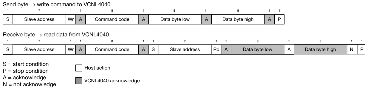
Fig. 12 - Write Word and Read Word Protocol
