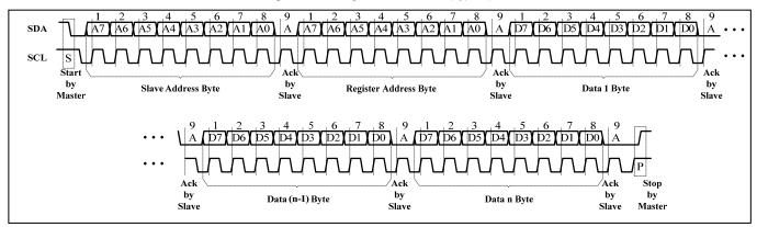
Figure 6 Writing to IS31FL3235A (Automatic Address Increment)
