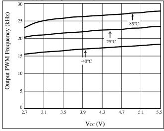
Figure 9 V<sub>CC</sub> vs. Output PWM Frequency
