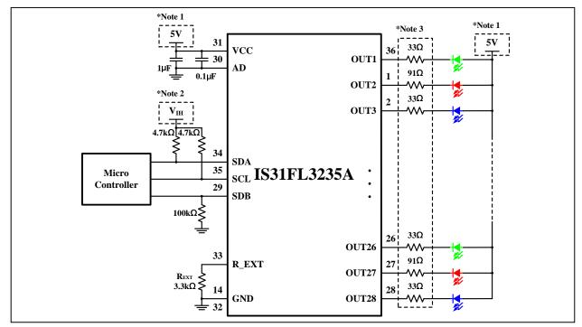
Figure 2 Typical Application Circuit (V<sub>CC</sub>=5V)
