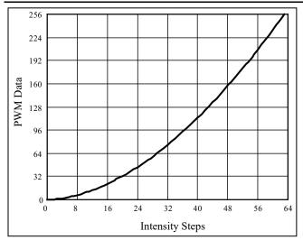
Figure 7 Gamma Correction (64 Steps)
