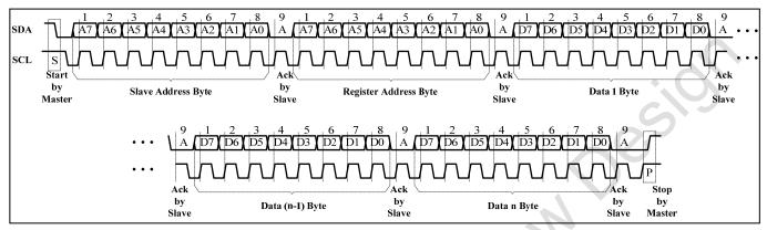
Figure 5 Writing to IS31FL3236 (Automatic Address Increment)
