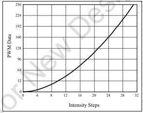
Figure 6 Gamma Correction (32 Steps)
