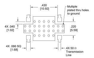
Dimensions are in Inches [Millimeters] XC0900A-05\* Mounting Footprint
