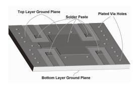
Figure 2: Solder Paste Application
