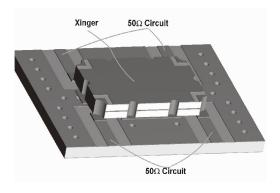
Figure 3: Component Placement
