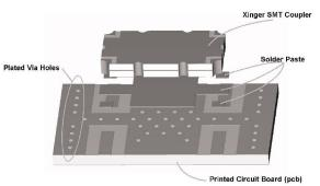
Figure 4: Mounting Features Example
