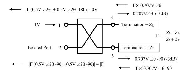
The reflection property of common mismatches in 3dB couplers is very beneficial to the operation of many networks. For instance, when splitter/combiner networks are employed to increase output power by paralleling transistors with similar reflection coefficients, input return loss is not degraded by the match of the transistor circuit. The reflections from the transistor circuits are directed away from the input to the termination at the isolated port of the coupler.
