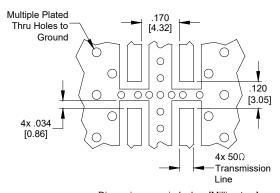
Dimensions are in Inches [Millimeters] XC0900P-03AS Mounting Footprint
