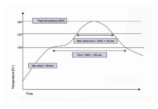
Figure 6 - High Temperature Solder Reflow Thermal Profile
