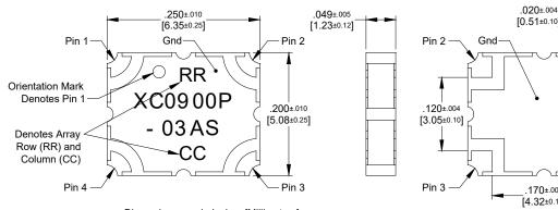
Dimensions are in Inches [Millimeters] XC0900P-03AS Mechanical Outline
