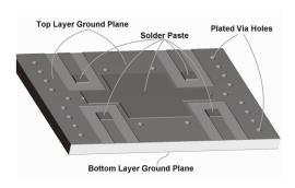
Figure 2: Solder Paste Application
