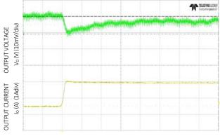
Figure 9. Typical output ripple and noise ( $C_0=2x47\mu F$  ceramic,  $V_{IN}=12V$ ,  $I_0=I_{O,max}$ ,).
