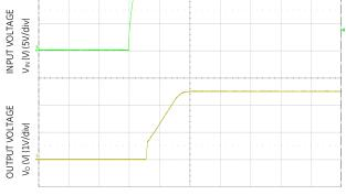
Figure 23. Typical Start-up Using On/Off Voltage ( $I_0 = I_{0,max}$ ).
