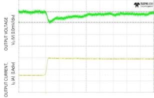
Figure 3. Typical output ripple and noise ( $C_0=2x47\mu F$  ceramic,  $V_{IN}=12V$ ,  $I_0=I_{0,max}$ ,).
