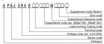
(Note1): PSJ series, 2.5V560μF (ESR 4m Ω max.) has supplement code "J". Terminal and terminal plating are the same as all other in PSJ series.
