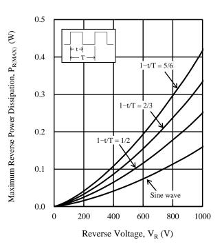
Figure 5.  $P_{R(MAX)}$  vs.  $V_R$  ( $T_J = 150 \ ^{\circ}C$ )
