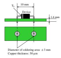
Figure 1. Lead Temperature Measurement Conditions
