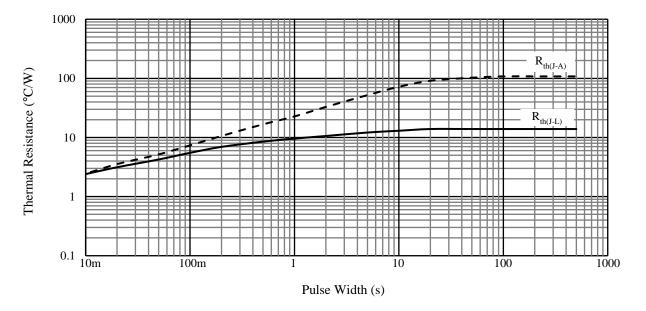
Figure 8. Typical Transient Thermal Resistance Characteristics
