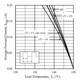
Figure 2.  $I_{F(AV)}$  vs.  $T_L^{(2)}$  ( $T_J = 150 \ ^{\circ}C, V_R = 0 \ V$ )
