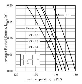
Figure 3.  $I_{F(AV)}$  vs.  $T_L^{(2)}$  ( $T_J = 150 \text{ °C}$ ,  $V_R = 1000 \text{ V}$ )
