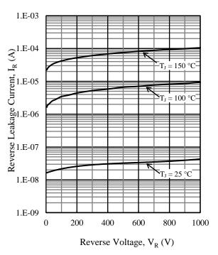
Figure 7. Typical Characteristics: I<sub>R</sub> vs. V<sub>R</sub>
