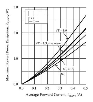
Figure 4.  $P_{F(MAX)}$  vs.  $I_{F(AV)}$  (T<sub>J</sub> = 150 °C)
