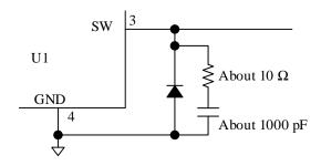
Figure 12-11. SW pin peripheral circuit
