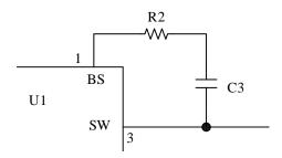
Figure 12-10. BS pin peripheral circuit
