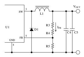
Figure 12-16. FB pin peripheral circuit
