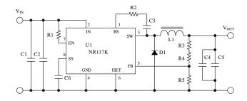
Figure 12-1. The IC Peripheral Circuit
