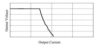
Figure 11-7. Output Voltage Characteristics at Overcurrent
