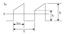
Figure 12-5. Current Waveform of Input Capacitor
