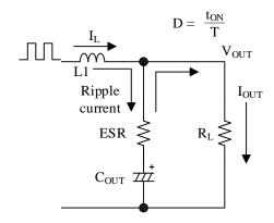
Figure 12-6. Current Flow of Output Capacitor
