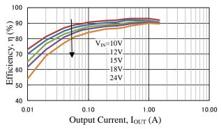
Figure 5-1. Efficiency ( $V_{OUT} = 3.3 \text{ V}$ )
