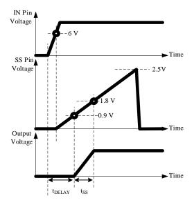
Figure 11-3. Soft Start Operation Waveform
