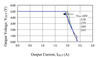
Figure 5-3. Output Startup (Load = CR)
