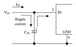
Figure 12-4. Current Flow of Input Capacitor
