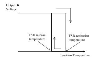
Figure 11-8. Output Voltage Characteristics of Thermal Shutdown
