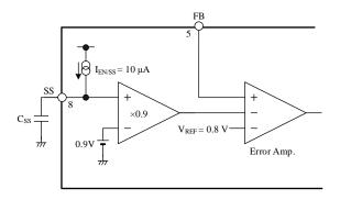
Figure 11-2. SS Pin Internal Circuit
