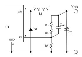
Figure 12-8. Using Electrolytic Capacitor
