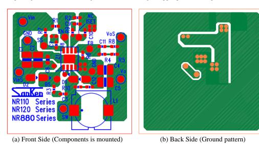
Figure 13-1. Pattern Layout Example (PCB size: 40 mm × 40 mm)
