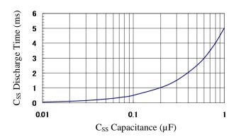
Figure 11-4. C<sub>SS</sub> Discharge Time vs. C<sub>SS</sub> Capacitance
