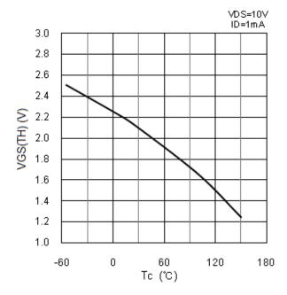
Figure 14.  $V_{GS(TH)}$  vs.  $T_C$
