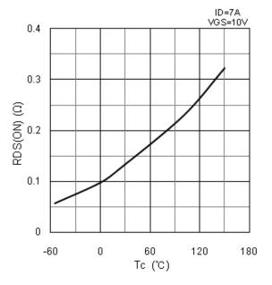
$Figure \ 9. \quad R_{DS(ON)} \ vs. \ T_C$
