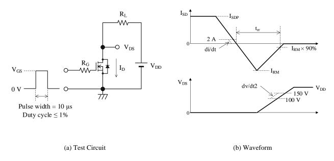
Figure 2. Diode Reverse Recovery Time Test
