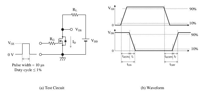
Figure 3. Resistive Load Switching Time Test
