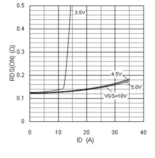
Figure 8.  $R_{DS(ON)}$  vs.  $I_D$
