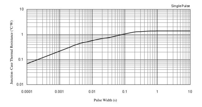
Figure 15. Transient Thermal Resistance Characteristics
