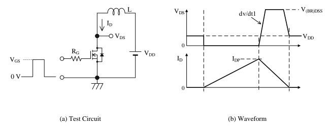
Figure 1. Unclamped Inductive Switching Energy Test
