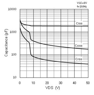
Figure 10. Capacitance vs.  $V_{DS}$
