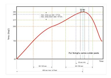
Fig 2. Infrared soldering profile
