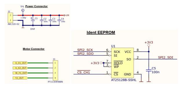
Figure 2: Motor connector, power connector and EEPROM
