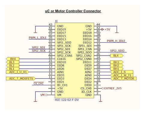
Figure 1: 44 pin Motor Controller Connector
