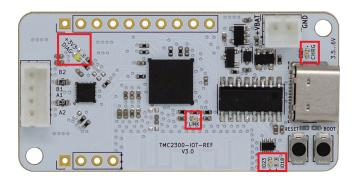
Figure 2: TMC2300-IOT-REF Onboard LEDs (indentical on V3.0 and V4.0 boards)
