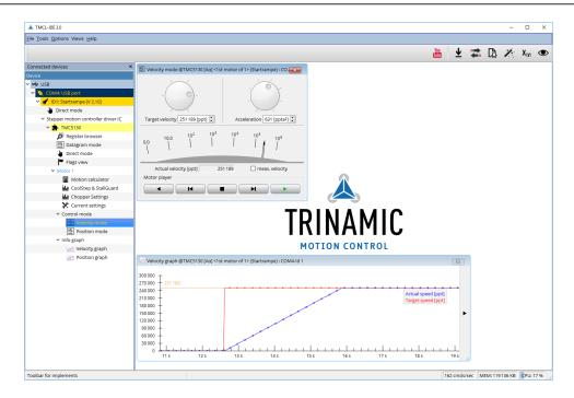
Figure 4: Driving the motor in velocity mode (TMCL-IDE provides similar view for TMC5031-EVAL)
